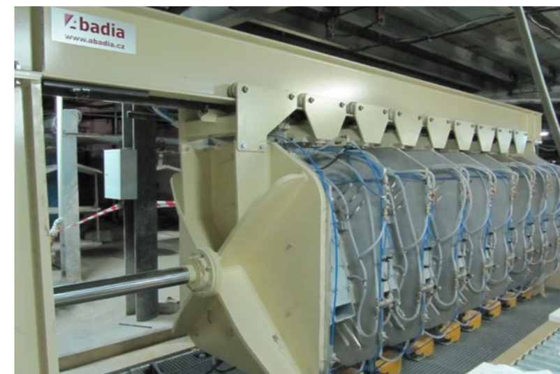
High pressure machine for casting of sinks, Kirov, Russia
